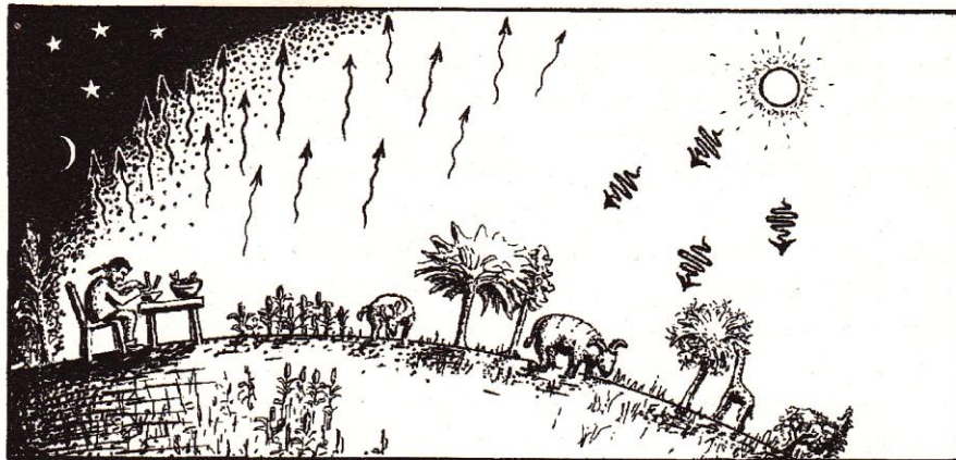
Fig. 27.9 The Earth gives back the same amount of energy that it receives from the Sun, but what it receives from the Sun is in a much lower entropy form, owing to the fact that the Sun's yellow light has higher frequency than the infrared that the Earth returns. Accordingly, by Planck's E = h\nu , the Sun's photons carry more energy per photon than do those that Earth returns, so the energy from the Sun is carried by fewer photons than that returned by the Earth. Fewer photons means fewer degrees of freedom and therefore a smaller phase-space region and thus lower entropy than in the photons returned to space. Plants make use of this low entropy energy in photosynthesis, thereby reducing their own entropy, and we take advantage of the plants to reduce ours, by eating them, or eating something that eats them, and by breathing the oxygen that the plants release. This ultimately comes from the temperature imbalance in the sky that resulted from the gravitational clumping that produced the Sun.
