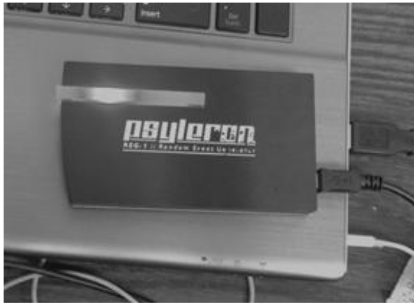
Figure 2. Random event generator (REG); Psyleron REG-1 device used throughout the following experiment
