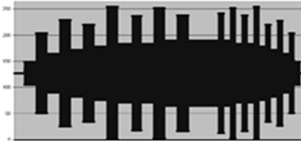
Figure 1. Waveform image of GMA-patterned field repeated over the course of each exposure; the y-axis is waveform point value (equivalent to voltage value between -5 to +5 V), the x-axis is time
