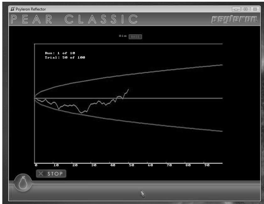
Figure 5. Screenshot of Reflector software collecting data from REG device; jagged center line is the moving cumulative deviation
